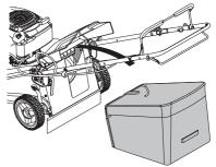
3 Release the back shield and allow it to rest on top of the grass bag frame.
