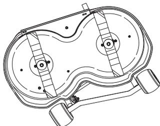
**IMPORTANT!** One or more unbalanced blades, caused by damage or poor balancing after sharpening, can cause vibrations in the machine.
