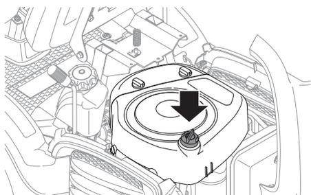
The dipstick should be **completely screwed down**
