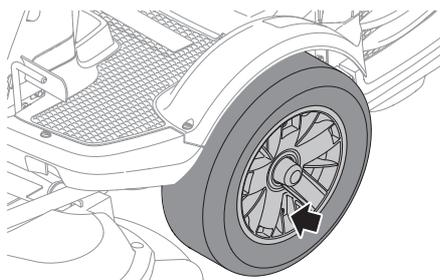
CAUTION! Different tyre pressures on the front tyres will result in the blades cutting the grass at different heights.
