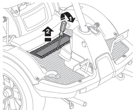
To put back the cover, it must first be bent and inserted at the sides. Then press down the cover.
