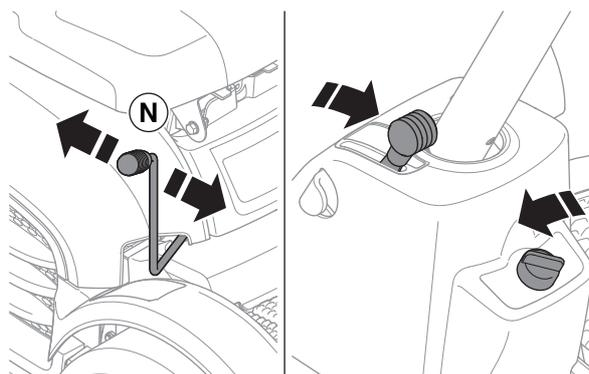
When the ride-on mower is at a standstill, engage the parking brake.
