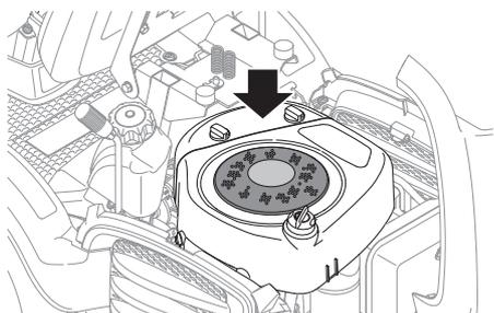
A blocked cooling intake will interfere with the cooling of the engine, which can damage the engine.
