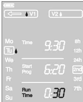
Each valve can be **opened or closed manually at any time**. A program-controlled open valve can also be closed early without changing the program data (watering start time, watering duration and watering frequency). The controller must be fitted.
