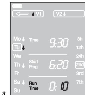
3. Whilst the watering time in minutes is flashing, the watering duration can be modified with the ▼-▲ button (between 0:00 and 0:59) (example: 10 minutes) and confirm with the OK-key.
