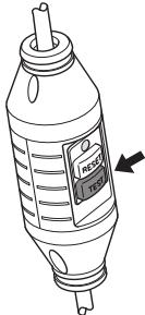
The ground fault circuit interrupter should trip and the machine switch off instantly. If not, contact your dealer.
