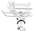
Recommended settings: Bar 13"-15": Minimum flow Bar 16"-18": Medium flow Bar -20": Maximum flow
