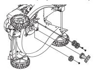
Remove belt from blade adapter / engine pulley and idler assembly.
