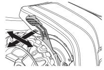
· The adjuster lever is spring loaded.
