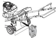
2 Close the back shield to allow the machine to discharge material to the left of the machine while cutting.
