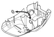
For running the machine in cold weather or powder snow, a special cover is available, which is mounted on the starter housing. This reduces the intake of cold air and prevents large amounts of snow from being sucked in.
