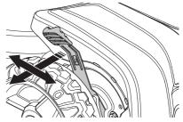
• The adjuster lever is spring loaded.
