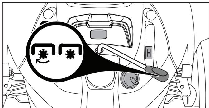
(☒) LE LEVIER D'EMBAYAGE D'ATTACHEMENT "DÉBRAYÉE"
