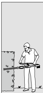
Side trimming: Telescopic pipe retracted
