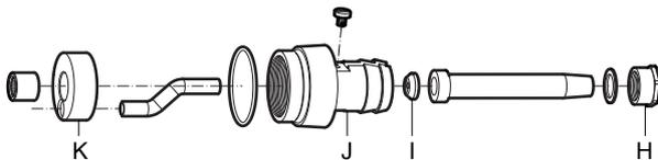
7. Use a suitable rod and a mallet to gently press the bearing holder (K) to remove the holder.
