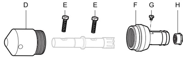
**NOTICE** Do not grease the inner shafts too extensively. Greasing too much can cause overload of the electric drive unit and trip the circuit breaker. Run the unit for two minutes continuously to distribute the grease in the flexible shaft before immersion in the concrete.
