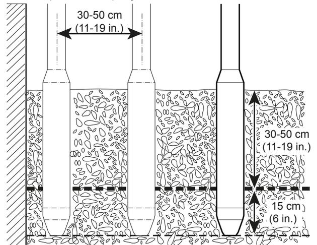
3. Insert the poker vibrator vertically at a distance of 8-10 times the tube diameter between insertions.
