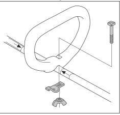
Make sure that the loop handle attaches between the arrows on the shaft
