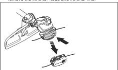
2. Pull out the line chute assembly
