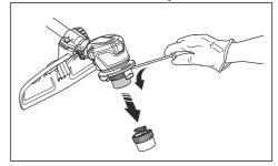
Remove the nut that holds the trimmer head and the drive disc.
