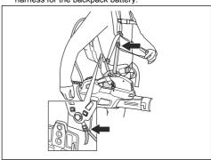
2. Adjust the harness to optimize the work position.
