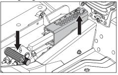
The cutting height pedals release the deck lift and set the desired deck height. Apply pressure to the lift pedal (lower) and rotate foot to also apply pressure to the release pedal (upper), unlocking the deck lift.
