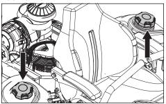
Read the safety instructions before refueling. The capacity for each tank is 22.7 litres (6 gallons). Regularly check the gas cap gasket for damage and keep the cap properly tightened.
