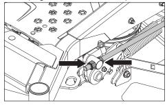
6. Be sure to check the previously measured distances to ensure that the mower deck is properly adjusted. The outer blade tip height must be equal when side-to-side. The rear blade tips must be 3.2 mm to 9.5 mm (1/8" to 3/8") higher than the front blade tip measurements when front-to-rear.
