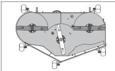
Measure and record the distance from ground to the bottom of the outer blade tip closest to the outside edge of the deck. Repeat this procedure for the other side. If the measurements are not the equal, adjustment is required. NOTE: Deck height adjusters are located on both the left and right sides of the mower deck. For illustration purposes, only the left side is shown.
