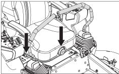
The seat can be adjusted lengthways with the lever located at the right hand side of the seat. When making adjustments the lever is moved upward.
