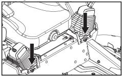
If the mower is not tracking straight, check the air pressure in the two rear tires. Recommended air pressure for the rear tires is 103 kPa / 1 bar / 15 psi.
