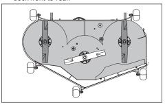
5. To set the front-to-rear deck height, adjust the locknuts on the threaded adjustment rods. Raise or lower the deck until the rear blade tips are positioned 3.2 mm to 9.5 mm (1/8" to 3/8") higher than the front blade tips.
