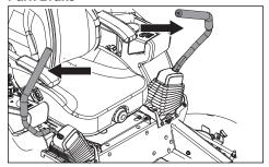
The park brake is integrated with the steering control levers. Move the two levers out from the neutral position to engage the park brake.
