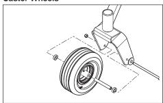
Check every 200 hours. Check that wheels rotate freely.
