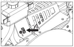
The fuel shut-off valve is located at the right rear of the seat. The valve has three positions: right tank, left tank and OFF.
