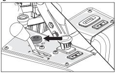
The ignition switch is used to start and stop the engine. On models equipped with headlights, turn the key clockwise to ACCESSORY for headlight use.
