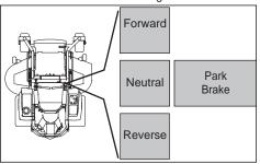
Zero turn can be achieved by moving one control backward (behind the neutral position) and carefully moving the other steering control forward from its neutral position. The rotation direction when zero turning is determined by which steering control is moved backward behind the neutral position. If the left steering control is pulled backward, the machine turns to the left. Use more care when using this maneuver.
