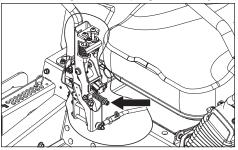
To change the park brake tension, tighten the pivot bolt until the desired braking is correct.
