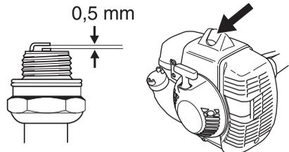
**CAUTION!** Always use the recommended spark plug type! Use of the wrong spark plug can damage the piston/cylinder. Check that the spark plug is fitted with a suppressor.
