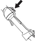
**CAUTION!** The stop switch automatically returns to the start position. In order to prevent unintentional starting, the spark plug cap must be removed from the spark plug when assembling, checking and/or performing maintenance.
