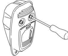
If the muffler on your machine is fitted with a spark arrestor mesh this must be cleaned regularly. A blocked mesh will cause the engine to overheat and may lead to serious damage.
