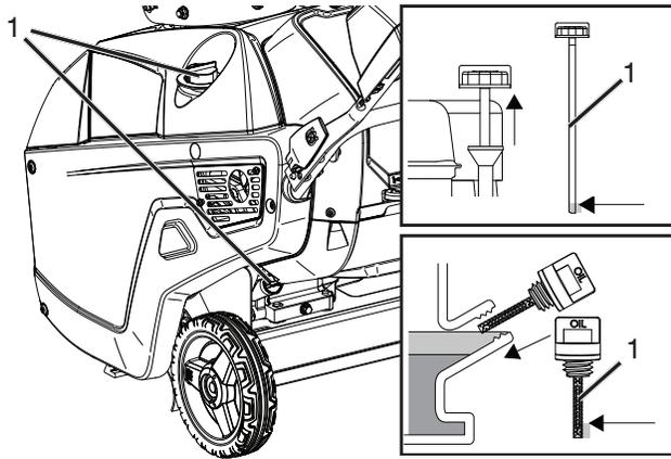
4. Insert the dipstick into the filler neck and turn clockwise until fully seated. Then remove the dipstick by turning it counter-clockwise.
