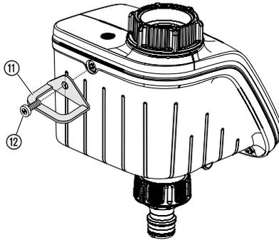
1. Screw clamp ⑪ with screw ⑫ firmly to the back of the Water Control.
