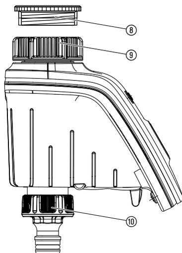
The Water Control is fitted with a sleeve nut ⑨ for taps with (G 1") (33.3 mm) thread. The adaptor supplied ⑧ allows the Water Control to be connected to taps with a (G 3/4") (26.5 mm) thread.
