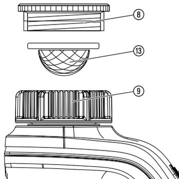
The filter ⑬ should be checked regularly and cleaned when necessary.
