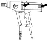
Use compressed air to periodically clean the motor. Remove the inspection cover and clean the cover.
