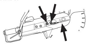
Unscrew the nuts and lift off the front belt guard.
