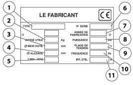
1. Type 2. Weigth 3. Maxi tool 4. Bore 5. Speed 6. Serial 7. Fabrication year 8. Power 9. Voltage 10. Frequency 11. Intensity
