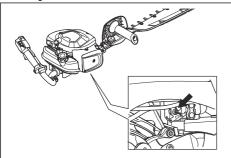
Turn the idle adjustment screw counterclockwise until the cutting attachment stops.
