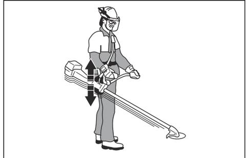
5. If the operation is to cut grass, let the cutting attachment stay lightly on the ground. Adjust the harness clamp to balance the product correctly.
