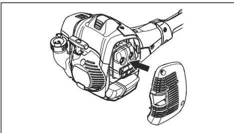
3. Remove the screw holding the spark arrestor mesh.
