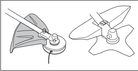
1. Make sure that the cutting attachment guard is not damaged or cracked.
