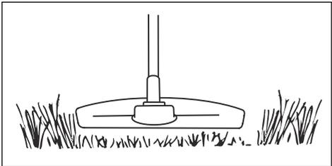
2. Do not push the trimmer head to the ground. This can cause damage to the product.
