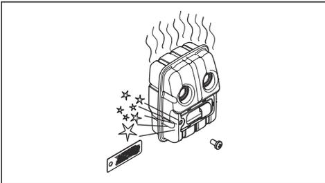
4. Clean the spark arrestor mesh if it is blocked or replace it if it is damaged.
