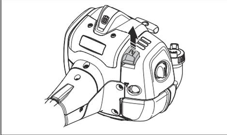
2. Remove the air filter cover and remove the air filter.
