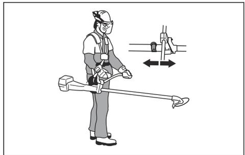
For grass clearing, the product is correctly balanced when the blade is at cutting height near the ground.
