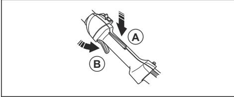
2. Make sure that the throttle control is locked at the idle setting when the throttle trigger lockout is released.
