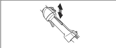
4. Do a check of the throttle control and throttle trigger lockout move freely and that the return springs work properly.
