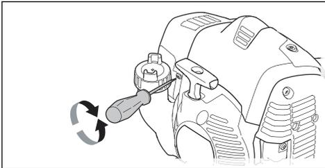
3. Turn the idle adjustment screw clockwise until the cutting attachment starts to turn.
