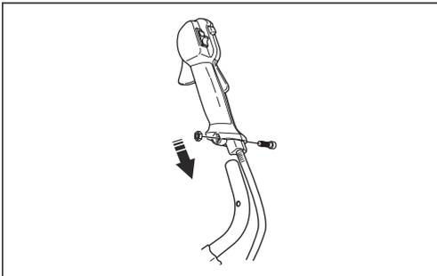
2. Align the hole on the throttle handle with the hole in the handlebar.
