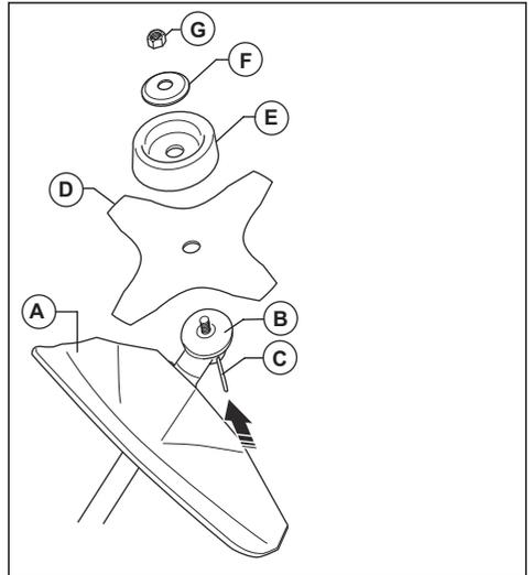
2. Turn the output shaft to align 1 of the holes in the drive disc (B) with the related hole in the gear housing.
