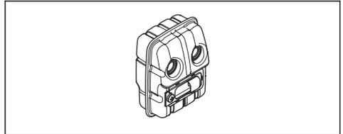
The muffler keeps noise levels to a minimum and sends exhaust fumes away from the operator.
