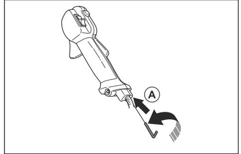
4. If the start throttle speed is too high, turn the adjuster screw (A) counterclockwise until the cutting attachment stops. Turn the adjuster screw (A) clockwise 1/2 turn more.
