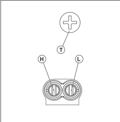
Turn the H-jet and L-jet clockwise to get less fuel in the mixture and counterclockwise to get more fuel in the mixture. Less fuel in the mixture gives a higher engine speed and more fuel in the mixture gives lower speed.
