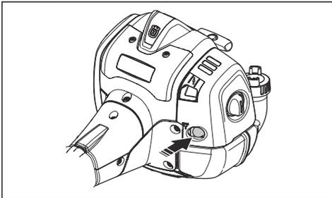
2. Move the choke control up into choke position.
