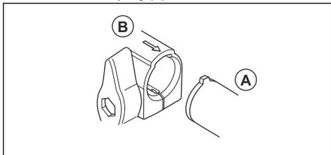
3. Carefully push the shaft into the coupling until you hear a click.
