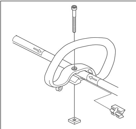
2. Install the spacer into the slot of the loop handle.
