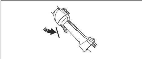
3. Press the throttle trigger lockout and make sure that it returns to its initial position when you release it.
