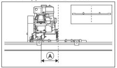
Tighten the screws (A). Torque to 68 Nm.
