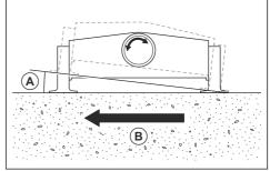
Move the product forward (B) at a speed of 0.5– 1.0 m/min. or 1.6–3.2 ft/min.
