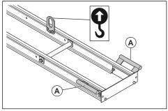
If you use lifting equipment, attach the lifting equipment to the lifting eyes.
