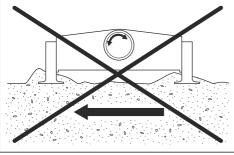
**Note:** If the height of the concrete is more than 20 mm/0.8 in., the product becomes too heavy to pull and the concrete surface behind the product is not smooth. If the height of the concrete is less than 10 mm/0.4 in., the vibrations do not give a good result.
