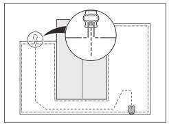
a) Put the 2 ends of the boundary wire and the end of the guide wires into the coupler.
