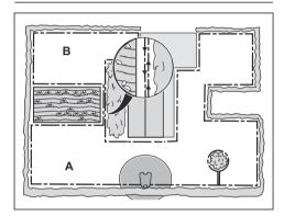
Put the boundary wire around the secondary area (B) to make an island. Refer to To make an island on page 18.
