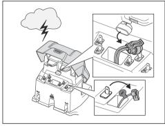
To reduce the risk of damage to electrical components in the product and the charging station, we recommend that all connections to the charging station are disconnected (power supply, boundary wire and guide wire) if there is a risk of a thunderstorm.
