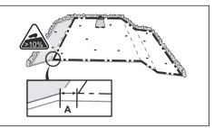
For slopes adjacent to a public road, put a barrier of minimum 15 cm / 6 in. along the outer edge of the slope. You can use a wall or a fence as a barrier.
