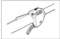
2. Set the choke control to the choke position.
