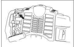
b) Turn the idle speed screw T counterclockwise until the cutting attachment stops.
