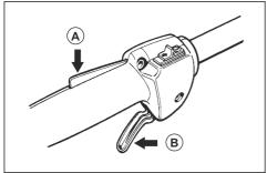
2. Release the throttle trigger lockout and make sure that the throttle control is locked at idle speed.
