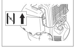
Push the air purge bulb until fuel starts to fill the air purge bulb.
