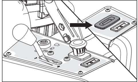
The service meter is located on the left hand control panel and shows the total operating time with the blades engaged.
