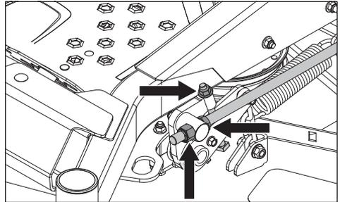
3. Turn the two outer blades to align with the deck front to rear. Reposition the rear blade mounting bolts up or down until the rear blade tips are positioned 1/8" to 3/8" (3.175 mm - 9.525 mm) higher in the rear than the front blade tips.
