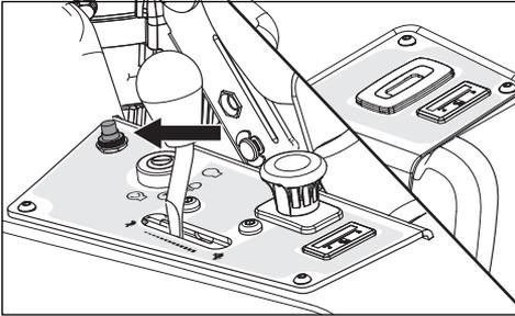
The Malfunction Indicator Light (MIL) blinks to warn when sensors detect an engine system problem. Refer to the engine manufacturer's owner's manual for detailed instructions on determining the type of malfunction and the appropriate steps for repair.
