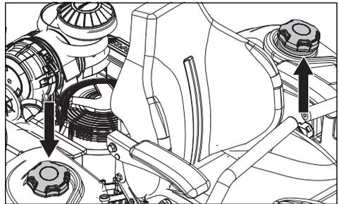
Read the safety instructions before refueling. The capacity for each tank is six gallons (22.7 liters).
