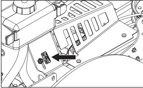
The fuel shut off valve is located at the right rear of the seat. The valve has three positions: right tank, left tank and OFF.
