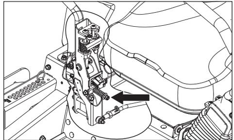
3. To change the park brake action, tighten the pivot bolt until the desired braking feel is correct.
