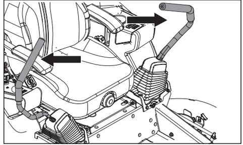
The park brake is integrated with the steering control levers. Move the two levers out from the neutral position to engage the park brake.
