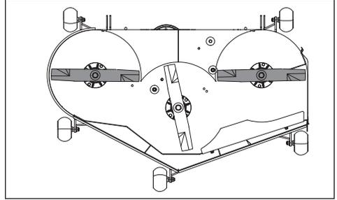
2. Measure from the floor surface up to the bottom of the blade tip on the discharge side of the mower deck. Record this measurement. Move to the opposite side; check that measurement is the same. If adjustment is required, loosen the locknut and adjust the bolt up until the two side to side measurements are equal. Retain measurement.
