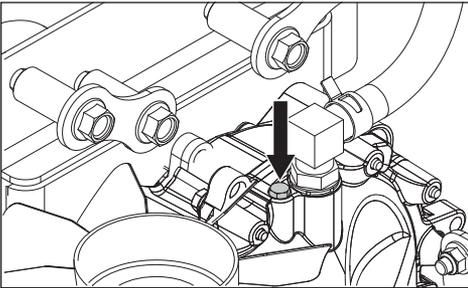
8. Fill with 20W50 motor oil until the oil appears at the bottom of each transaxles' top port, approximately 2 quarts (1.89 liters) per transaxle, 4 quarts (3.78 liters) total.
