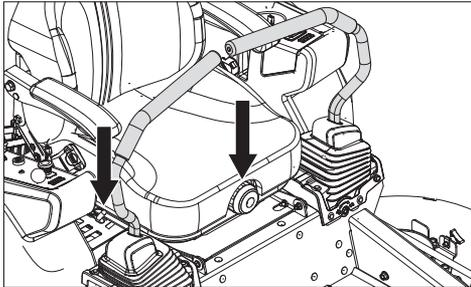
The seat can be adjusted lengthways with the lever located at the right hand side of the seat. When making adjustments the lever is moved upward.
