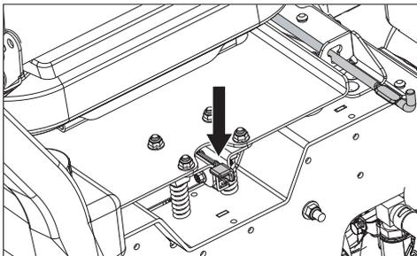
The seat can be rotated forward to access the mower battery and hydro gears. Push down on the latch lever to release the seat. Raise the seat until the rod engages.
