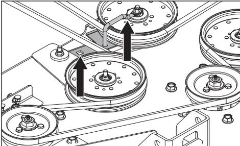
4. With a 1/2" breaker bar and using the square opening in the idler arm, shift the arm counter clockwise to relieve the tension on the belt.
