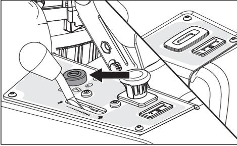
The ignition switch is used to start and stop the engine. On models equipped with headlights, turn the key clockwise to ACCESSORY for headlight use.
