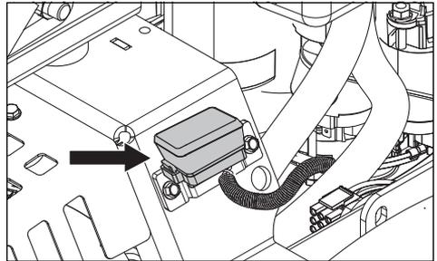
Fuses are located on the left hand side of the machine and are accessed by tilting the seat forward. Fuses are flat pin fuses type as used in automobiles. The 20 A is the primary fuse. The 7.5 A is for the mower deck coupling. The 10 A is for accessories.
