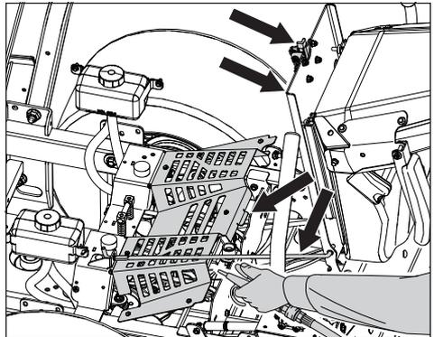
4. Blow off debris accumulated around the transaxle pump and fans.
