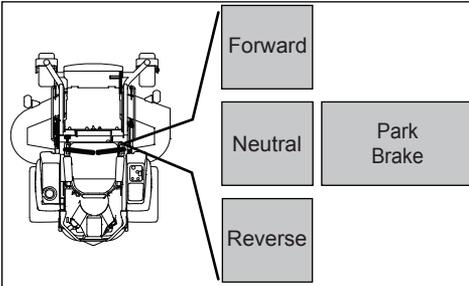
Zero turn can be achieved by moving one control backward (behind the neutral position) and carefully moving the other steering control forward from its neutral position. The rotation direction when zero turning is determined by which steering control is moved backward behind the neutral position. If the left steering control is pulled backward, the machine turns to the left. Use more care when using this maneuver.
