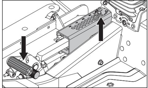
The cutting height pedals release the deck lift and set the desired deck height. Apply pressure to the lift pedal (lower) and rotate foot to also apply pressure to the release pedal (upper), unlocking the deck lift.
