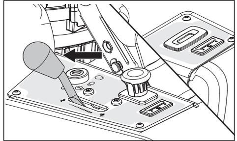
The throttle control regulates the engine speed and the rate of rotation of the blades, assuming the blade switch is pulled out.
