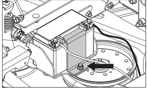
3. Using two wrenches, disconnect the BLACK battery cable then the RED battery cable.
