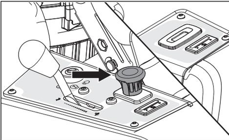
To engage the mower deck, pull the knob out; mower blades are disengaged when the knob is pressed down.
