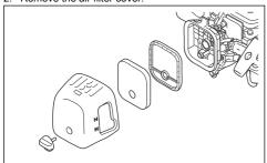
3. Remove the felt filter and the air filter.
