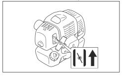
Hold the product to the ground. Pull out the cord slowly with your right hand until you feel some resistance. Pull the cord quickly and with force. Keep doing it until you hear the engine start.
