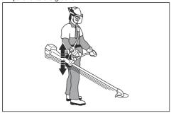
Let the cutting attachment stay lightly on the ground. Adjust the harness clamp to balance the product correctly.
