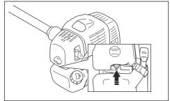
3. Set the choke control to the run position, then pull the start rope until the engine starts.
