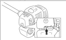
3. Move choke control to the choke position.
