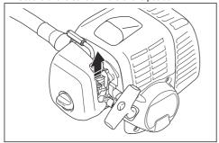
Hold the product to the ground. Pull out the cord slowly with your right hand until you feel some resistance. Pull the cord quickly and with force. Keep doing it until you hear the engine start.
