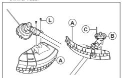
2. Attach the drive disc (B) and support flange (G) to the output shaft.
