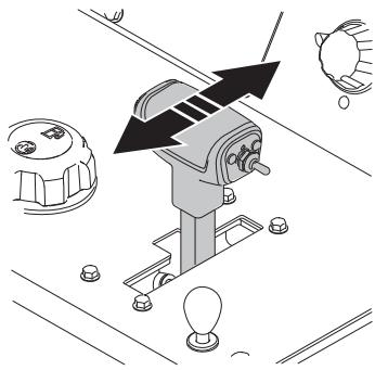
**WARNING!** Do not put transmission in neutral while the machine is parked on a grade or hill. The operator will lose control and injury or damage could occur.
