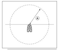
**Note:** The product uses the charging station signal to find the charging station when it is in the docking area.
