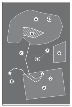
For a complete map installation, you must install a work area and a charging station on the map.
