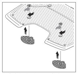
Put the 2 top baseplates on top of the lower baseplate.
