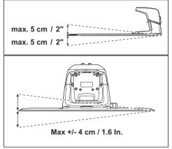
The baseplate of the charging station must not be bent.
