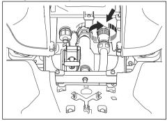
Lift the rear part of the cutting deck and tilt the lever.
