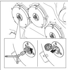
5. Loosen the screw with the Combi tool.
