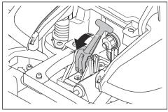
Push down the lever and lift up the front of the cutting deck by the handle. Make sure that the cutting deck is in a vertical position.
