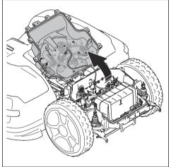
8. Disconnect the 2 cables from the battery.
