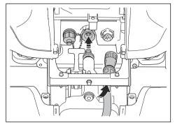
7. Align the shaft with the hole in the frame.
