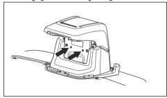
If the LED indicator lamps do not have a green light, do a check of the installation. Refer to LED indicator lamps on the charging station on page 42 and To install the charging station on page 17.
