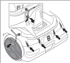
Remove the wheel cover with the flat screwdriver on the Combi tool. Clean the body of the product, wheels and chassis with a brush, compressed air or running water.
