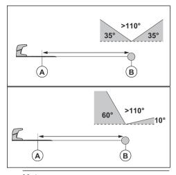
**Note:** Short reversing distance decreases the risk of track marks. A long reversing distance can be necessary to have good satellite signals at the docking point.
