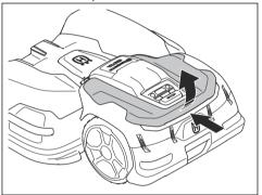
Loosen the clips with the flat screwdriver on the Combi tool and remove the rear bumper.
