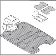
Attach the top baseplates to the lower baseplate with 6 couplings. Use a 8 mm hex key to attach the couplings.
