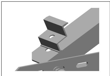
1. Install upper edge bracketing to both sides then install the lower edge bracketing to both sides
