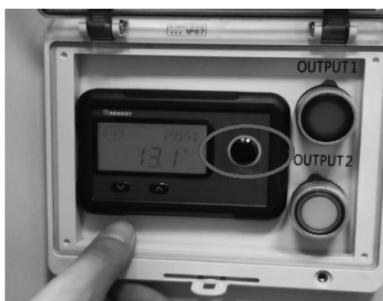
**NOTE** The two output buttons next to the monitor are for turning on and off the charging station outputs.
