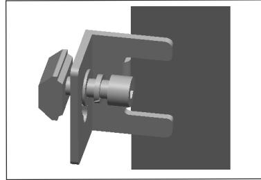
Use (x2) Part A (brackets) and slide horizontally through both sets of channel nuts at top & bottom.
