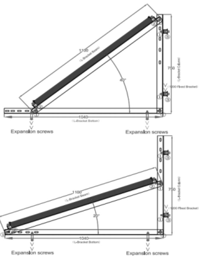
1. >M8X25 Cap Screw + Flange Nut + Lock Washer + Flat Washer
