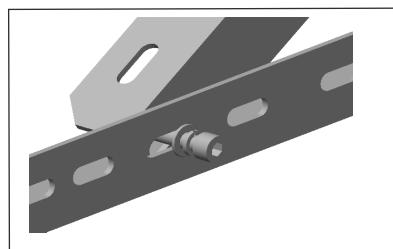
Connect the two triangle ends together using the (x2) Part (A) Bracket.
