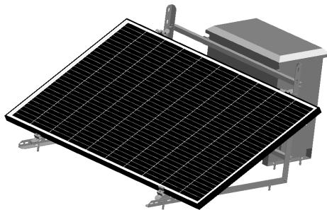
Once the panel is secure, plug in the solar panel via the attached MC-4 connectors into the MC-4 connectors coming out of the enclosure ( Male > Female, Female > Male).
