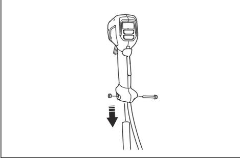
2. Move the throttle handle to the right side of the handlebar.
