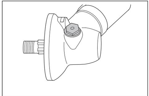
4. Look into the grease plug hole and turn the drive shaft. The grease level (A) must be in level with the top of the gear cogs (B).
