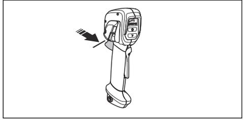
2. Press the power trigger and make sure that it goes back to its initial position when you release it.
