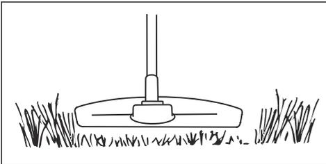
2. Do not push the trimmer head to the ground. The ground and the product can be damaged.
