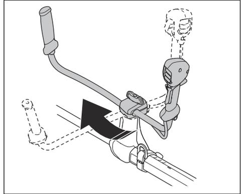
3. Turn the handlebar around the shaft until the handlebar clamp locks into transport position.
