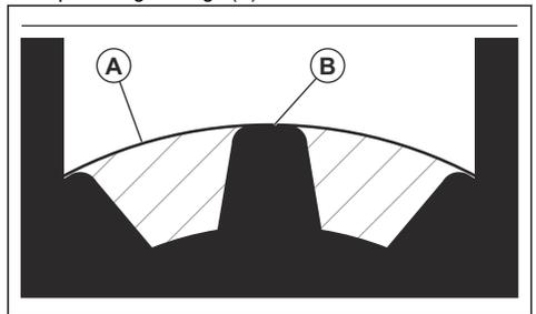
5. If the grease level is too low fill the bevel gear with Husqvarna bevel gear grease. Fill slowly and turn the drive shaft as you apply the bevel gear grease, stop at the correct level (B).
