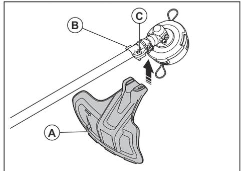
2. Install the cutting attachment guard on the shaft and tighten it with the bolt (C).
