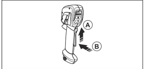
3. Make sure that the power trigger and the lock moves freely and that the return spring operates correctly.
