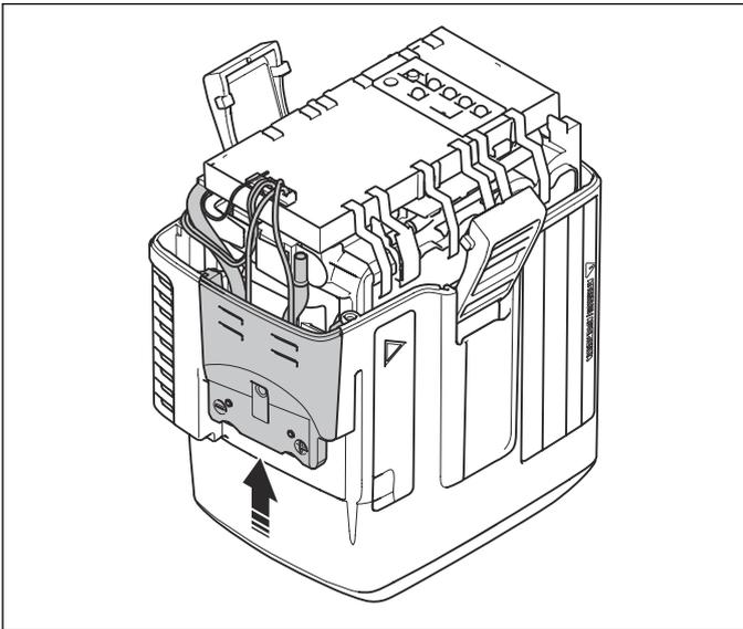
8. Remove the battery pack. Hold the battery pack at the ends of the circuit board to prevent short circuit.
