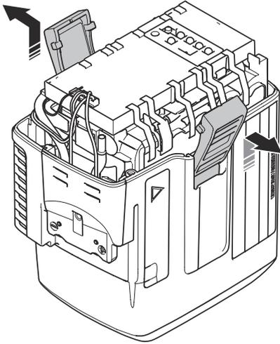
7. Push out the battery connector from the slot.
