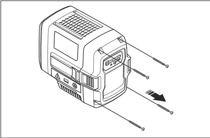
4. Put the screws at a safe distance from the battery.
