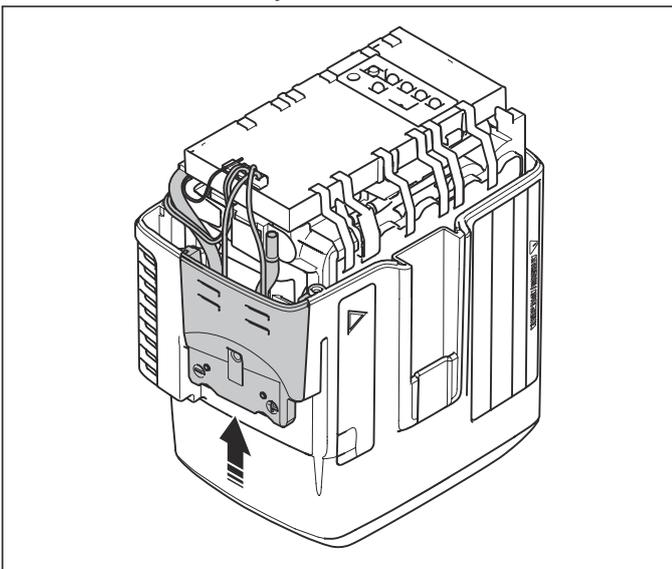
7. Remove the battery pack. Hold the battery pack at the ends of the circuit board to prevent short circuit.
