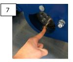
When the drive-motor and wheel are aligned, the quick release pin will lock into place. Close wheel guard.
