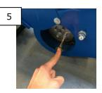
!WARNING! Use **only 1 finger** to press the button of the quick release pin, and keep applying pressure.
