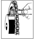
On mounting coupling links with springs, their closed sides should point to the running direction of the chain (see figure). Put the spring onto the link plate and press it over the pin into the ring groove by means of a pair of tongs. Demount the spring in the opposite order.
