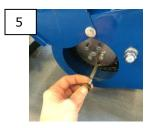
Insert the quick release pin inside the hole.
