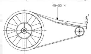
When the belt can be pressed in by hand 5 - 10mm, it has the correct tension. (At  $\pm$ 10 kg pressure)
