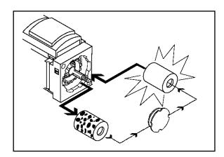
Fasten the filter screw and place the filter bowl back . Make sure the locking pin points towards the large
