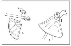
5. Remove the cutting attachment guard (A).
