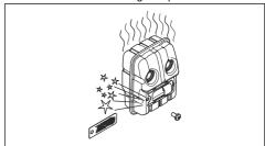
Clean the spark arrestor mesh if it is blocked or replace it if it is damaged.
