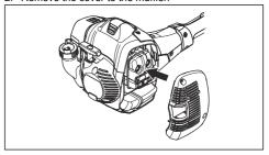
Remove the screw holding the spark arrestor mesh.
