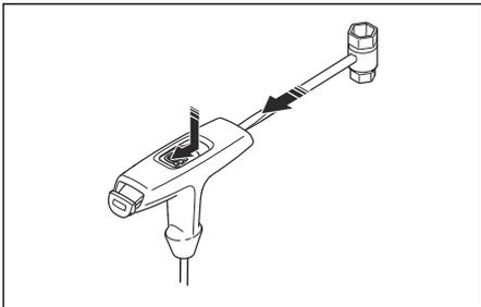
2. Turn the starter pulley approximately 2 turns clockwise.
