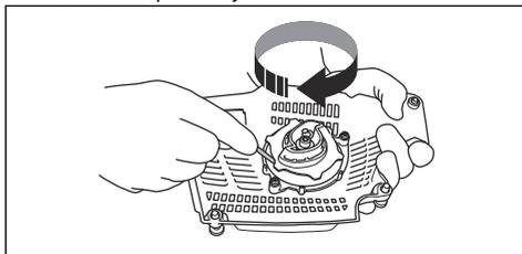
8. Attach a new starter rope to the pulley. Wind the starter rope approximately 3 turns around the pulley.
