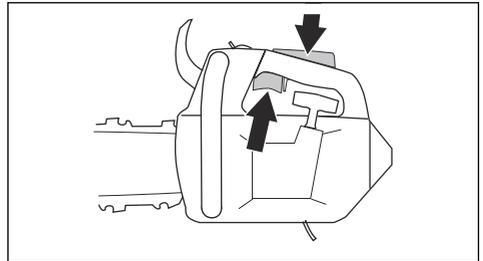
2. Push down the throttle trigger lockout and make sure that it goes back to its initial position when you release it.
