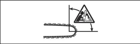
Kickback always occurs in the cutting plane of the guide bar. Usually, the product is thrown against the operator but can also move in a different direction. It is how you use the product when the kickback occurs that causes the direction of the movement.
