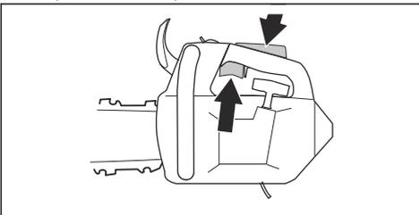
7. Move the front hand guard rearward to disengage the chain brake.
