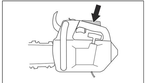
3. Make sure that the throttle trigger is locked at the idle position when the throttle trigger lockout is released.
