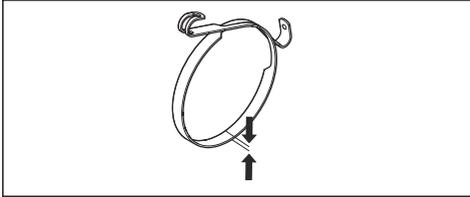
2. Do a check of the brake band. The brake band must be at a minimum of 0.6 mm/0.024 in thick at its thinnest point.
