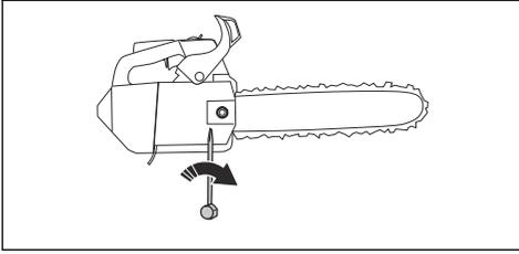
5. Tighten the bar nuts using the wrench and lift the front of the guide bar at the same time.
