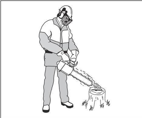
4. If the saw chain lubrication does not operate correctly, do a check of the guide bar. Refer to *To do a check of the guide bar on page 27* for instructions. Speak to your servicing dealer if the maintenance steps does not help.
