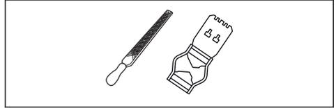
1. Use a flat file and a depth gauge tool to adjust the depth gauge setting. Only use Husqvarna depth gauge tool to get the correct depth gauge setting and bevel for the depth gauge.
