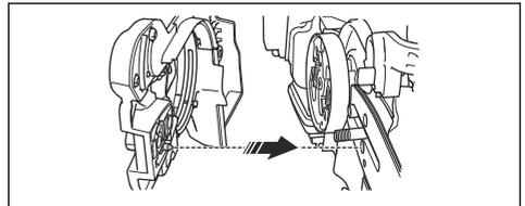
7. Tighten the bar nut finger tight.
