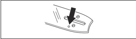
2. Examine if there are burrs on the edges of the guide bar. Remove the burrs using a file.
