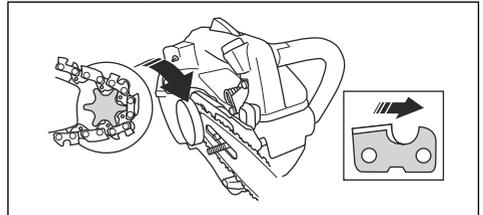
6. Align the hole in the guide bar with the chain adjuster pin and install the clutch cover.
