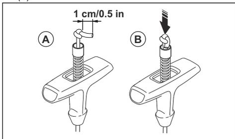
15. Pull the starter rope until 1 cm of the spring guide is shown. At the same time, assemble the starter handle cover.
