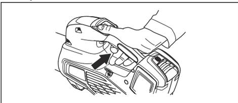
2. Press the cruise control button to set the chosen airflow, the LED comes on.
