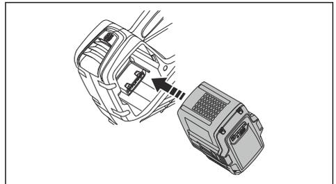
3. Press the lower part of the battery and push it in as far as it will go into the battery compartment. The battery will lock into position when you hear a click.
