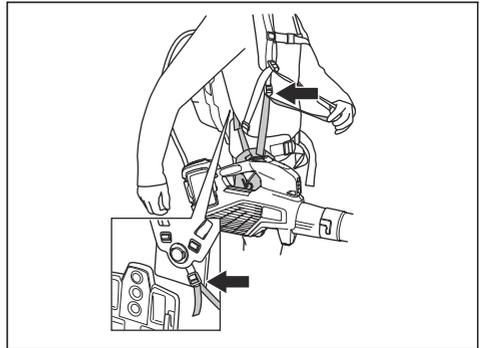
2. Adjust the harness to optimize the work position.
