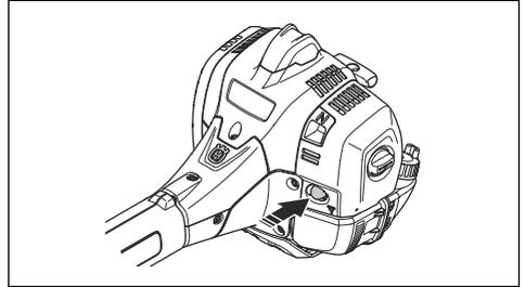
2. Pull the starter rope handle until the engine starts. Push the throttle trigger slowly to increase the speed gradually.
