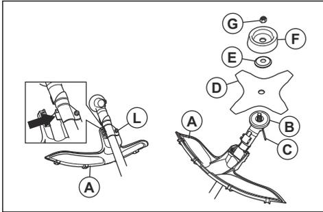
2. Attach the drive disc (B) to the output shaft.
