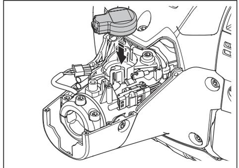
4. Install the connector to the Husqvarna connectivity device.
