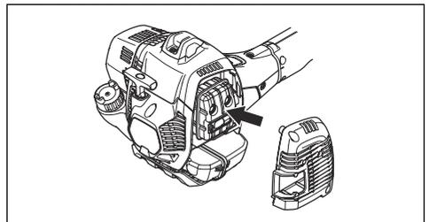
3. Remove the screw holding the spark arrestor mesh.
