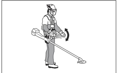
7. Tighten the handle adjustment knob fully.
