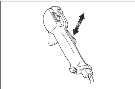
3. Make sure that the throttle trigger is locked at the idle position when the throttle trigger lockout is released.
