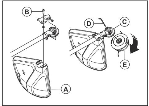
7. Turn the cutting equipment (E) in the opposite direction from which the cutting equipment rotate.
