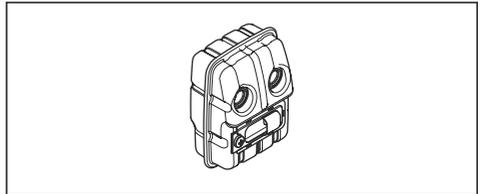
The muffler keeps noise levels to a minimum and sends exhaust fumes away from the operator.
