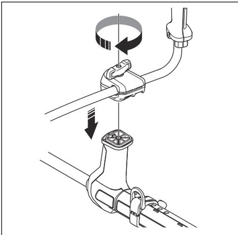
4. Tighten the handle adjustment knob slightly. Do not tighten the handle adjustment knob fully.
