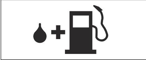
3. Shake the container and make sure that the fuel is fully mixed.
