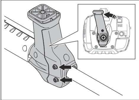
2. Put the handlebar bracket into position on the shaft. Tighten the 2 screws on the handlebar bracket.
