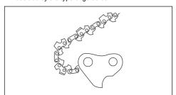
Bar groove width, in/mm. The groove width in guide bar must be the same as the chain drive links width.
