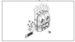
Clean the spark arrestor mesh if it is blocked or replace it if it is damaged.
