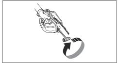
4. Tighten the saw chain until it is tight against the guide bar but still can move easily.
