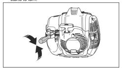
Turn the idle adjustment screw counterclockwise until the saw chain stops.
