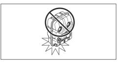
The muffler keeps noise levels to a minimum and directs exhaust fumes away from the operator. In areas with a hot, dry weather there is a high risk of fire. Obey local regulations and maintenance instructions
