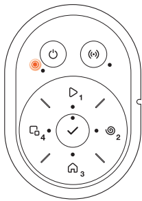
Charging or Standby
