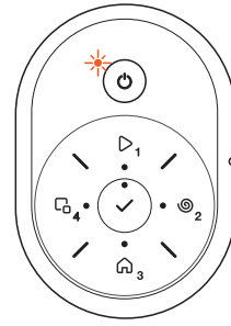
Charging or Standby
