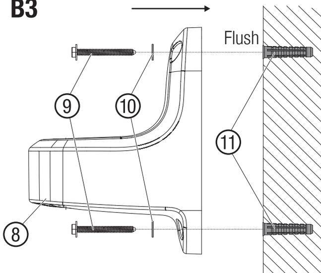
For most installations including wood, stucco, masonry and concrete, use hardware components ⑨, ⑩ and ⑪\*.
